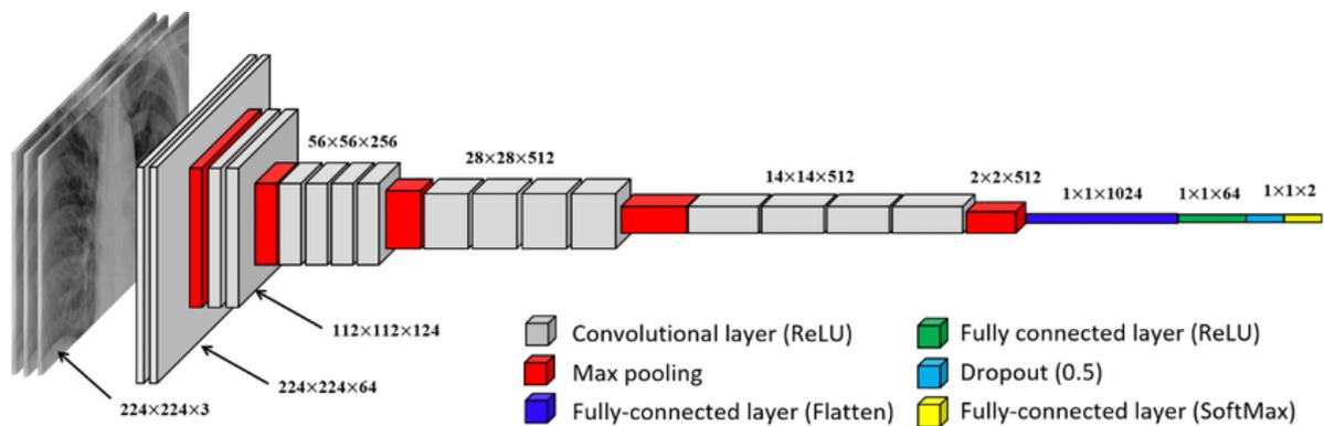
Figure 3: Architecture diagram of VGG19 model.
